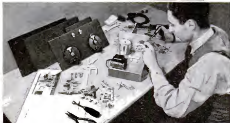
The converter in use. All ultrahigh-frequency tuning is done with dials of the converter set
